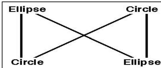
On the left of Figure 14, Circle is represented as a subtype of Ellipse, since a circle can be considered a special case of an ellipse in which both axes are equal. On the right is a representation that is sometimes used in object-oriented programming languages: Ellipse is considered a subclass of Circle, since it has more complex methods. If both ontologies were
